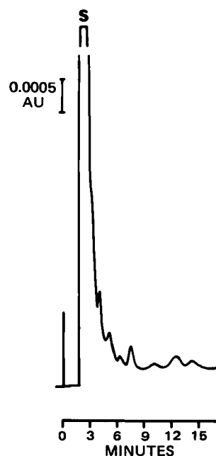
Figure 6 —Lung tissue following 35-min perfusion with an unsupplemented Krebs perfusate was homogenized, deproteinized with 0.6 N perchloric acid, and extracted on a C-18 disposable column (see text). Mobile phase used was 20% methanol in 0.1 M \text{KH}_2\text{PO}_4 -1 mM (\text{CH}_3)_4\text{NOH} . Other chromatographic conditions are as described under Experimental.
